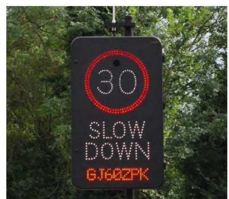
Figure 3 – Example of a Vehicle Activated Sign with ANPR
